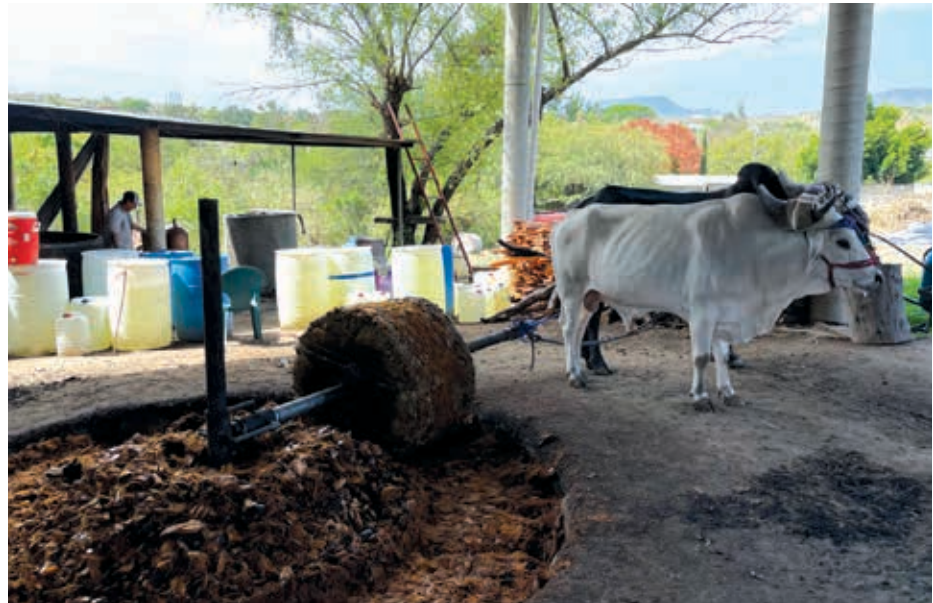
Some mezcal produced in Mexico involves a tahona, a large cement wheel pulled by a cow, horse or donkey, in a circle to mash agave hearts. Photo by Eric Timmerman.
