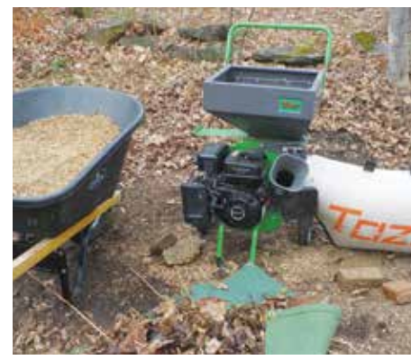
This gas-powered chipper-shredder helps make mulch and compost materials. Photo by Henry Homeyer.
