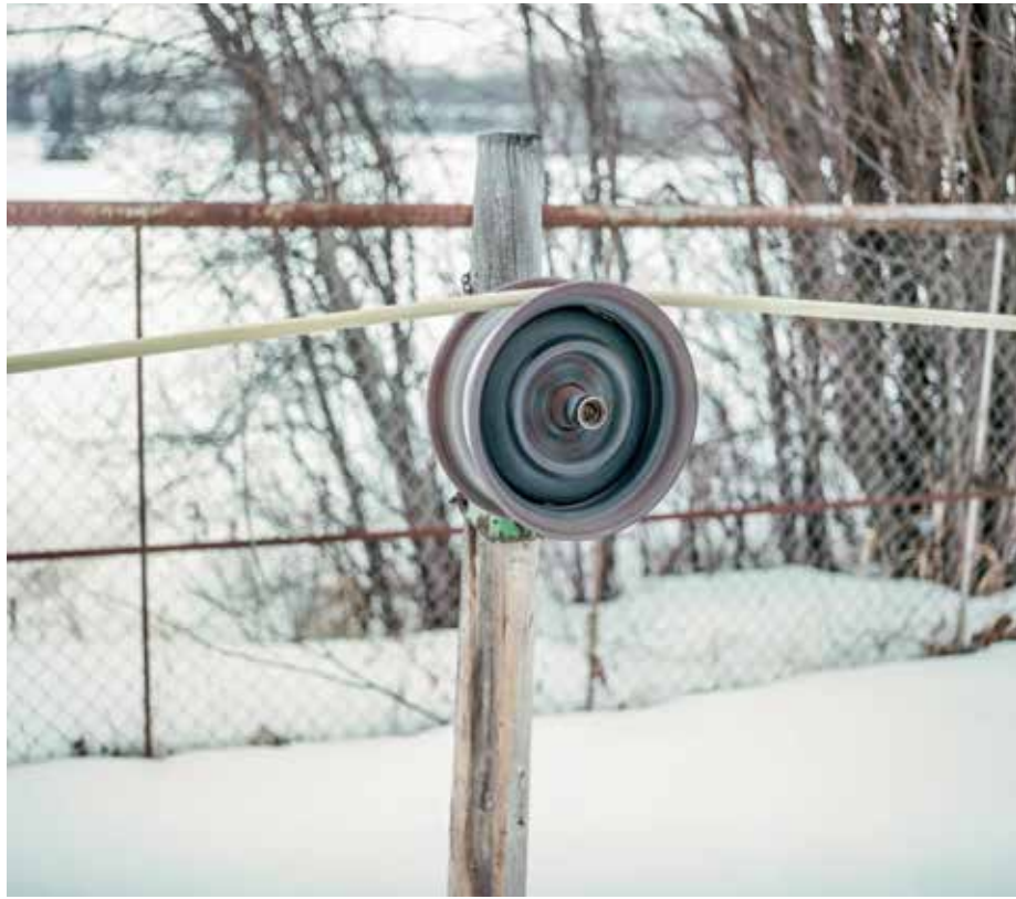
Modern rope systems employ high-tech lightweight rope and low-friction conveyance wheels. Photo courtesy of Rope Tow Operators Report.
