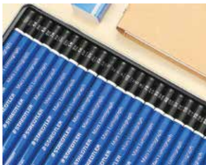
Pencils come in a variety of hardness, from very hard to very soft. The hardness is indicated with a number and letter system you'll find stamped on the pencil shaft. The 10H pencil is the most hard, while the 12B is the softest. Sketching sets usually provide pencils in a range of hardness, although not all have every grade. Softer grades are preferred by many artists for general purpose sketching and finished drawings.
